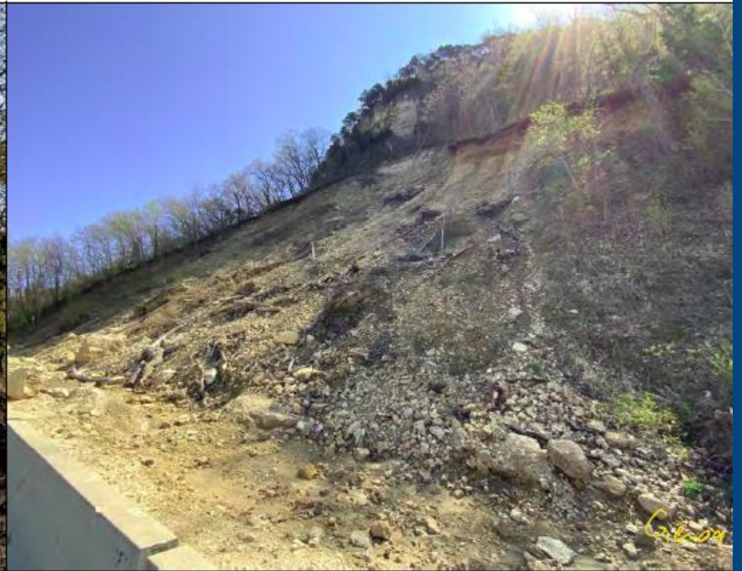
Shallow colluvial slides in the upper colluvium and lower colluvium/Lone Rock Formation
